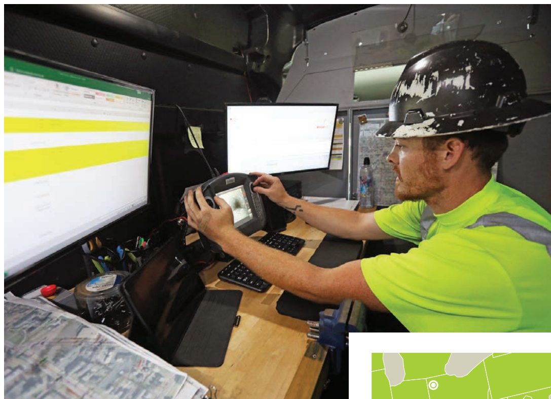
Technician Colton Roelfs monitors the progress of an Envirosight ROVER X camera during a sanitary sewer line inspection.
