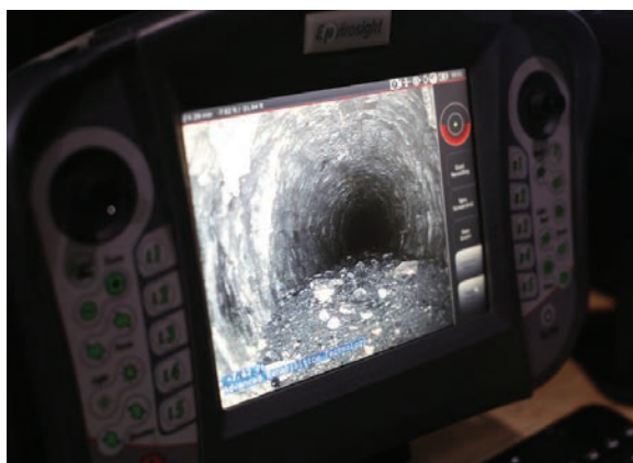
Technician Colton Roelfs monitors the progress of an Envirosight ROVER X camera during a sanitary sewer line inspection.
