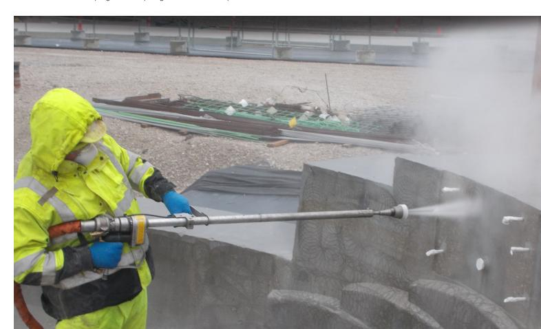
The two mockups had set outside from November through January freezing, thawing, and holding rain and snow. The pool material had several cracks appear in it, while the terrazzo over the polyurea was holding firmly. "I was allowed to take a hammer in front of our group and test the adhesion," remembers Mock. "It took several heavy blows, and even with that, it was the terrazzo that came off of the mortar bed before the mortar bed came off of the polyurea."
